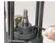
Packing gland is easily removed without special tools
